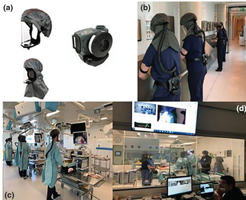
Fig. 1 Photographs showing (a) the two mask types (FH1 and FH2, both with soft-head cradles, neoprene chin seals and clear full-face visors with down-view panels certified to EN12941 TH3, EN166 1F) as well as PAPR use in simulated settings. Participants (b) scrubbing, (c) performing laparoscopic box tasks both individually and in pairs and (c) in full team operating room simulation.
